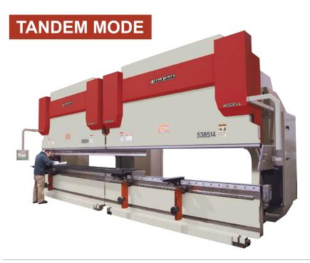
All Accell models can be installed in Tandem, where two or more machines operate as one. During operation, the machine controls are electronically connected to exchange information for fully synchronized forming.
