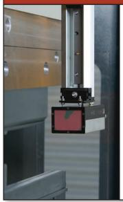
The Lazersafe Plus includes a dual beam system with a camera as a receiver that recognizes and monitors the silhouette of the punch. The Plus has the added benefit of allowing the ram to operate in fast speeds closer to the pinch point. This system is most efficient up to 18' ram/ bed lengths. A Sentinel Plus HL system is available for Accurpress models 20' and longer in length.
