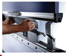
In addition to Crowing Systems, the Accell-E and U models include hydraulic Wila Ram Clamping Systems equipped to handle either American tang-style punches or Wila's large selection of New Standard tang-style punches. As a final complement, Accurpress offers a wide selection of press brake tooling. Choose from standard planner mill dies to high precision, including the complete Wila product line of ultimate exacting standards.
