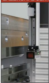
Lazersafe Sentinel is a Safety System offered on the Accurpress HT models that incorporates a continuous dual beam laser field protection zone directly below the punch tip. The Accurpress will immediately stop if any obstruction is detected when the ram is in motion. This system is most efficient up to 32' ram/bed lengths.
